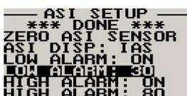
Enter the low airspeed set-point for when the alarm must activate. Any speed below this value will activate the alarm.
