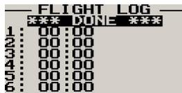
Select this function to view the flight log. The flight log contains the duration of each of the last 24 logged flights. Duration is displayed in hours and minutes. Eight flights are displayed at a time, Use the up/down or the rotary control to navigate through the log. Empty log entries are shown as "--:--".
