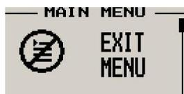
Pressing the rotary control on this menu item will cause the ASX-2 to exit the menu system. All changes made during navigation of menu system will be saved in non-volatile memory on exiting the menu system. If you remove power before exiting the menu the instrument will not save any changes.
