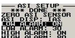
Select whether you want the low air speed alarm to be turned on or off. The low airspeed alarm is only activated once a flight has started.
