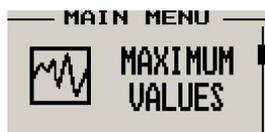
To avoid false recordings, the maximum values function is only activated 10 seconds after the instrument has powered up.
