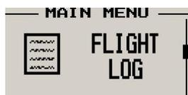
The ASX-2 uses the following algorithm to determine if a flight is in progress (Detect Mode): If airspeed is greater than the preset flight take off airspeed for the duration of 60 seconds or more, a flight is started with a logbook entry. The flight ends if airspeed falls below the preset flight take off airspeed for 30 continuous seconds. During a flight the logbook cannot be viewed.
